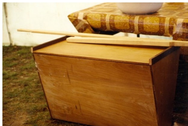
Mixing and rising bin with mixing paddle on top. 1992.
